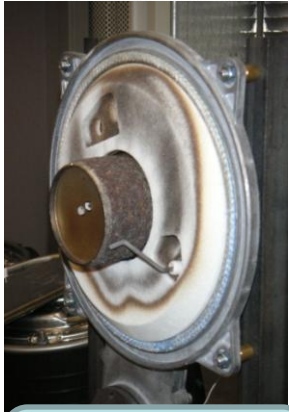
Low NOx Burner
